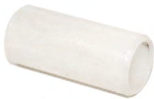
590004 Spring nylon bush ID 9/16" OD 3/4" L 45mm
