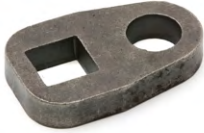
130003 Axle drop plate Drop: 3" Suits Stub: 39rd Suits Beam: 40sq Thickness: 25mm
