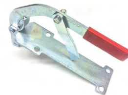
614055 Offroad coupling park lever brake plate suits Pin and Ball Couplings. Mounting detail: 4 hole Spacings: 184mm x 54mm Diameter: 13.5mm
