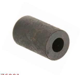
576301 Rocker Roller Spring steel bush 60mm wide, suits 16mm Pin
