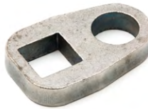
130009 Axle drop plate Drop: 3" Suits Stub: 45rd Suits Beam: 45sq Thickness: 25mm
