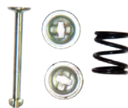
319017 Brake shoe hold down kit 9" hydraulic
