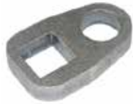
130007 Axle drop plate Drop: 3 1/2" Suits Stub: 45rd Suits Beam: 45sq Thickness: 25mm
