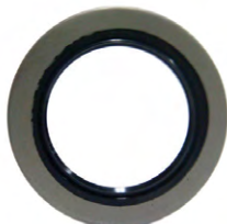
494015 Seal 610 - 2/2.5/3 Tonne. Suits nominal housing diameter: 89.96mm Seal Journal: 60.3mm
