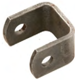
590442 Shallow Front Slipper Hanger 45mm spring 1/2" bolt
