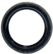
492015 Seal 610 - SL, Double lip Suits nominal housing diameter: 59.1mm Seal Journal: 43.9mm
