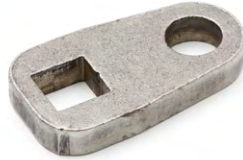
130004 Axle drop plate Drop: 4" Suits Stub: 39rd Suits Beam: 40sq Thickness: 25mm
