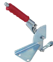
619150 Mechanical park brake mechanism, 280mm with cable pulley attached. Suits standard coupling rear fixing hole centres. May require 618926 to level coupling. Mounting detail: 2 hole Spacings: 55mm Diameter: 13mm
