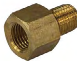
313003 Master cylinder adaptor 3/16" pipe. Use with copper washer between adaptor & master cylinder
