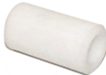
590002 Spring nylon bush ID 9/16" OD 7/8" L 45mm
