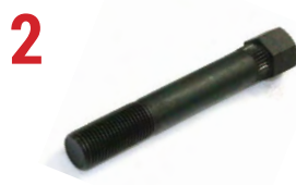
2 590608 Shackle pin 9/16" x 3 1/2" solid with 9/16" nyloc nut D 9/16" L 3 1/2"
