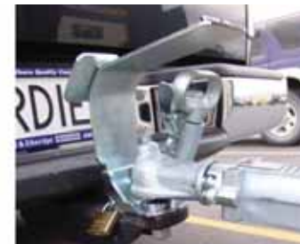
Bracket fitted removable wing slips into bracket used as security device
