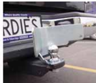
Removable wing slips into bracket
